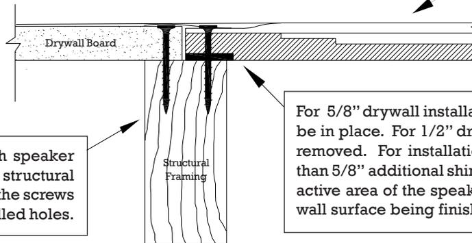
Both the drywall board and the Stealth speaker panel must be securely attached to the structural framing with drywall screws. Use all of the screws provided with the speaker in the predrilled holes.
